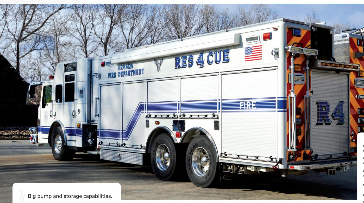
PUC<sup>™</sup> Heavy Duty Rescues minimize space used for fire suppression to maximize storage options – while still delivering 1,500 gpm with a single-stage pump.
